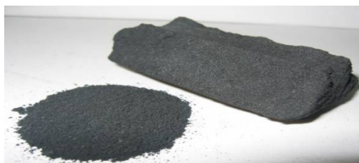
Fig 11 Activated carbon of IV value 1000 that is being used and mbs value about 350
